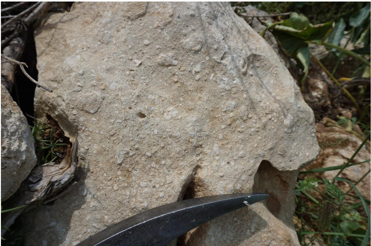
Outcrop Xb, marine inner shelf. Bioclastic limestone. 1: reworked red algae clasts
